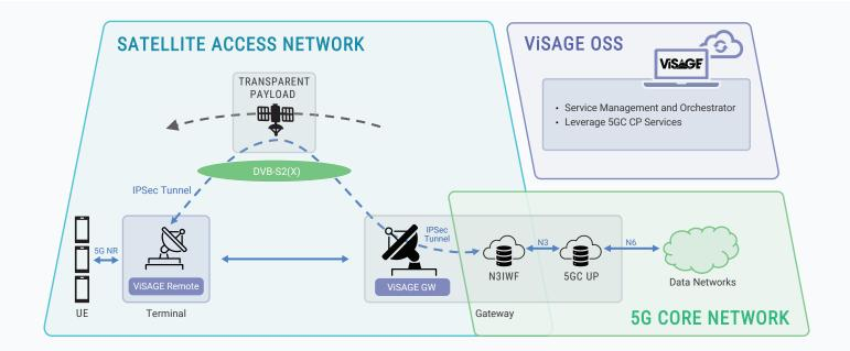
ViSAGE bridges the gap between SATCOM and 5G ecosystems to provide seamless, high-speed, low-latency connectivity. ViSAGE 3GPP-based 5G NTN OSS Platform and virtualized modem solution enable Satellite Network Operators and Ground Stations to access 5G service markets while digitising ground segment infrastructure.
